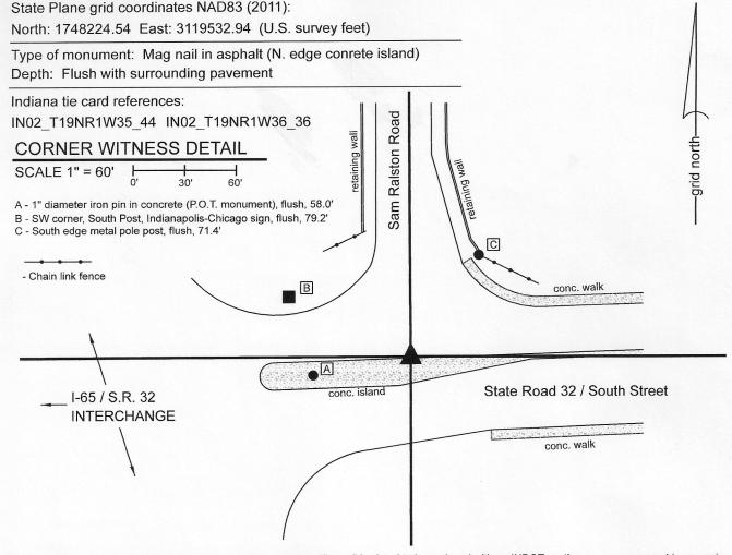
The Mag nail was found in place and held as marking the corner. The nail is slated to be replaced with an INDOT section corner monument in upcoming road work, per agreement with the INDOT Crawfordsville District Surveyor.
