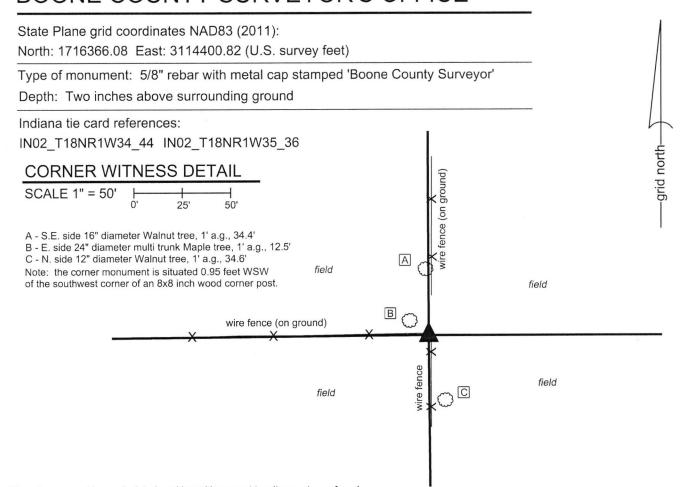
The rebar was set in a calculated position with respect to witness stones found.
