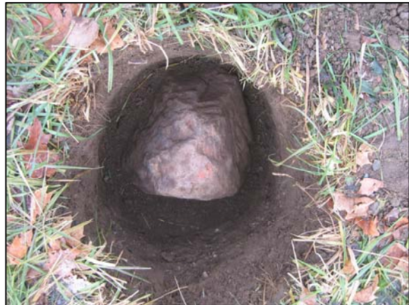
Close up of the closing corner stone with approximately 18 inches of the stone exposed.
