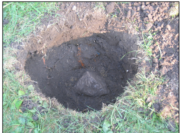
The lower stone found at corner 2 and the remains of the old wood post found adjacent to the two stones.
