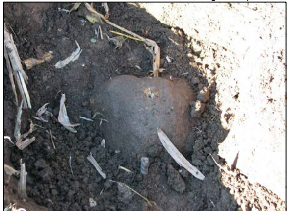
The stone with a hole drilled on top and a 5/8 inch rebar on the east side, no longer exposed.
