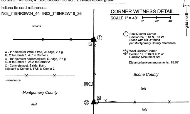
The stone marking Corner 1 (Montgomery County corner) was found per references provided by the Office of the Montgomery County Surveyor. The Harrison monument marking Corner 2 (Boone County corner) was set in place of a stone found.
