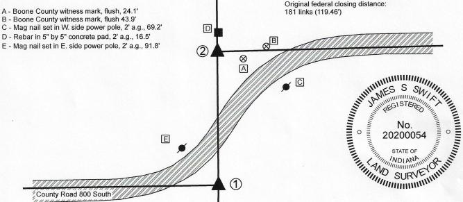
The stone marking Corner 2 was found in place and held as marking the
