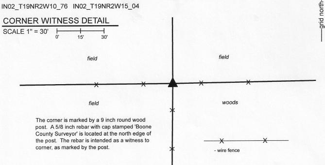
The 9 inch round wood corner post was found in place. The center of the post is held as the specific location of the corner. The rebar with "Boone County Surveyor' cap is intended as a witness to the corner.
