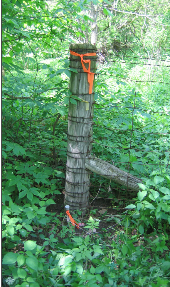
The post and rebar/concrete monument prior to excavation.
