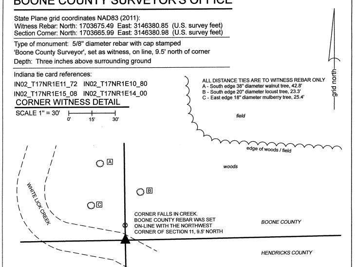
The witness rebar was set 9.5 feet north of a computed position of the corner.
