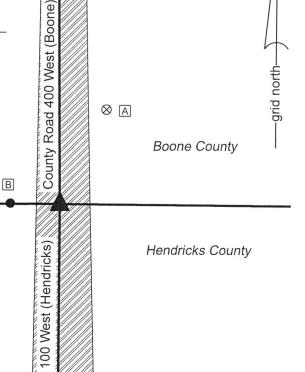
The Hendricks County monument, in the form of a 5/8 inch diameter rebar with metal cap over a stone, was found in place and held as marking the
