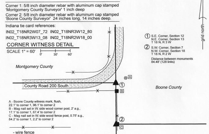
The rebar with metal cap was set at a calculated position.
