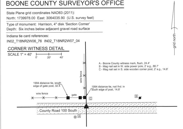
The Harrison monument was set in the position of a railroad spike, as perpetuated from a BCS tie card dated June 27, 1994. No specific descriptions of this corner were found in the BCS Surveyor's Record beyond the original establishment of the corner as a wood post in 1820 and a meaurement reference in an entry of 1834.
