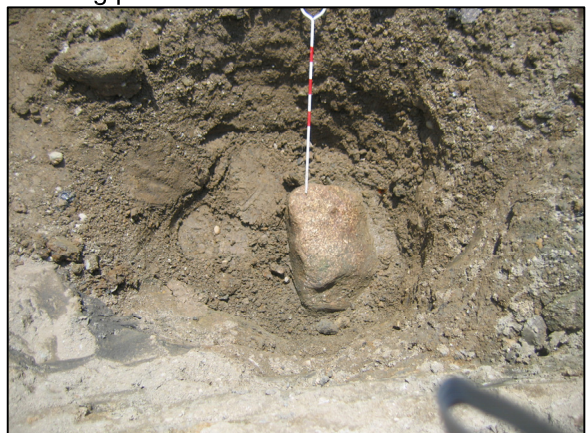
The lower record stone. The point of the chaining pin marks the etched mark on the stone.
