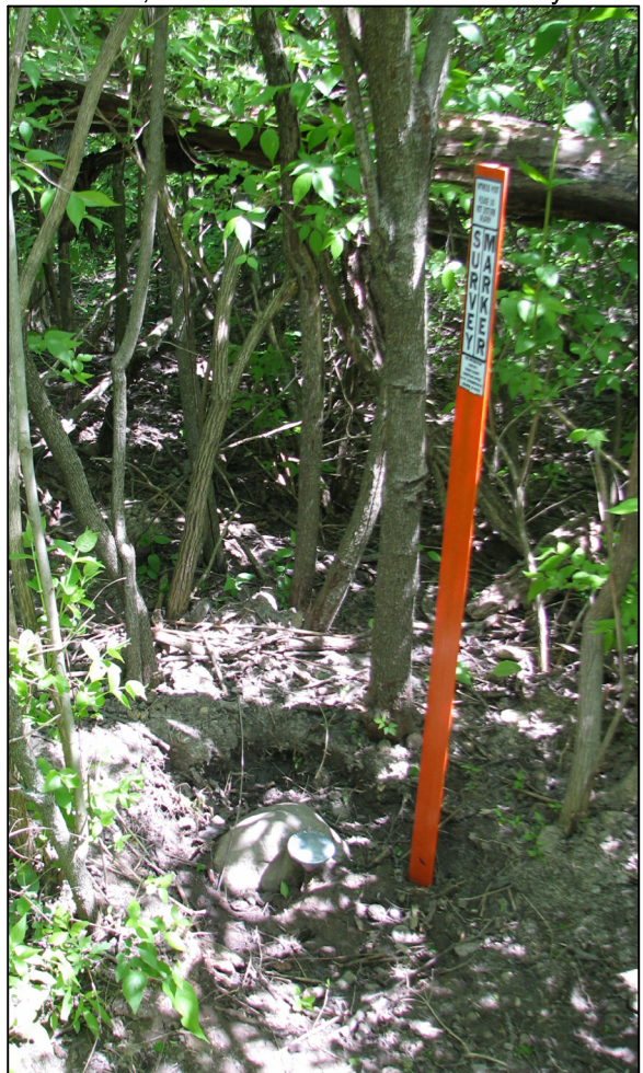
The stone, rebar and witness lathe on May 15.
