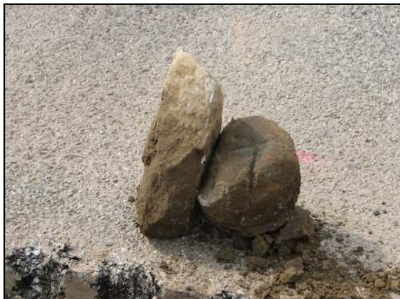
The stones removed from the road, oriented approximately as found below the road bed.
