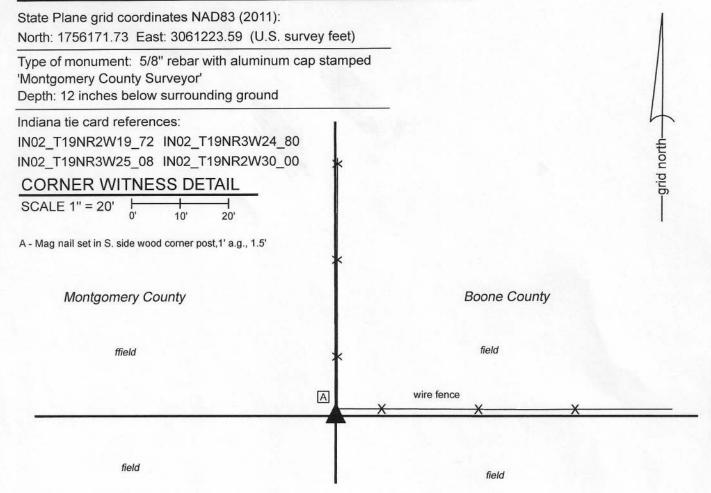
The rebar with Montgomery County Surveyor cap was found in place and held as marking the corner.
