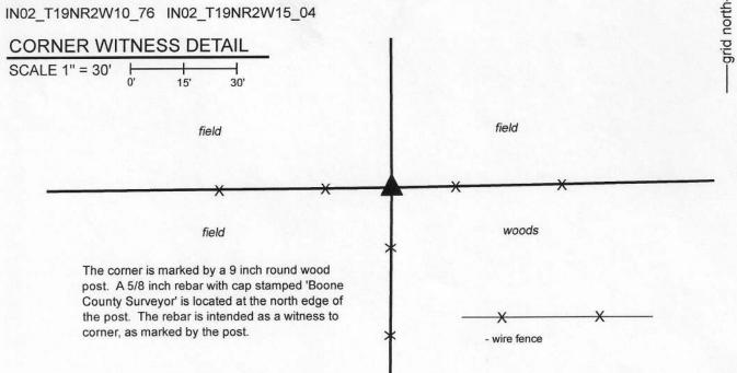
The 9 inch round wood corner post was found in place. The center of the post is held as the specific location of the corner. The rebar with "Boone County Surveyor' cap is intended as a witness to the corner.
