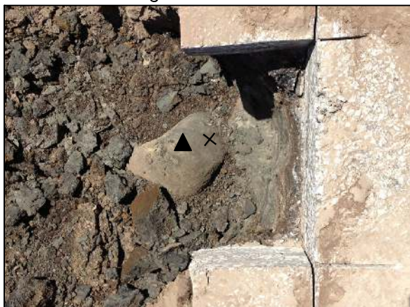
The same picture as is shown above. The etched "+" mark is enhanced for ease of visual detection and the high point is denoted with a black triangle.
