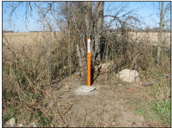
The harrison monument, set in place of the base of the old post and rebar.
