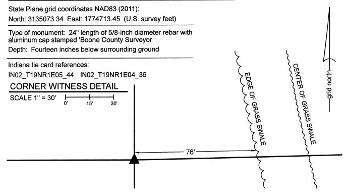
The rebar with Boone County cap was set at a calculated position.
