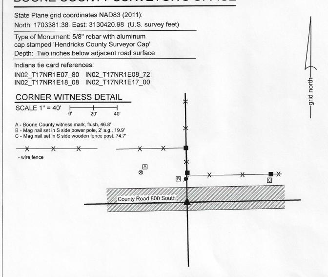
The rebar with Hendricks County Surveyor cap was found in place and accepted as marking the corner.
