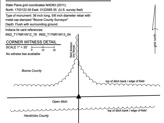
The rebar with Boone County cap was set at a computed position.
