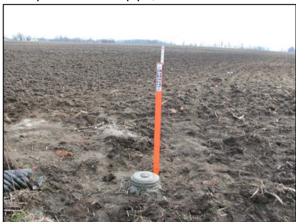
The harrison monument set within the concrete filled piece of storm pipe, View from the N.E.
