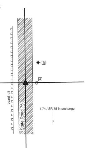
The INDOT Type B monument was found in place and held as marking the corner. A BCS tie card shows dated December, 2003 shows the corner as a railroad spike in the center of State Road 75 in line with an old fence to the west. Subsequently, the spike was removed and replaced with an INDOT Type B monument. No excavation was performed at this corner as it falls in a State Road and is also on the approach to the interchange of State Road 75 and Interstate 74.
