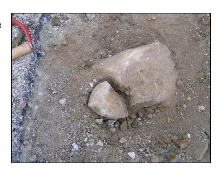
Photograph of the record stone, lifted to show etched "+" on west side. Photo is taken from the west. The stone had apparently been hit, the top broken off, and pushed over onto the west side. The dimensions of the stone match the record description. The stone was removed and the Harrison set over the position where the bottom of the stone was embedded in clay. The broken-off portion of the top is not shown in this photograph. The stone is on display in the Boone County Surveyor's Office.
