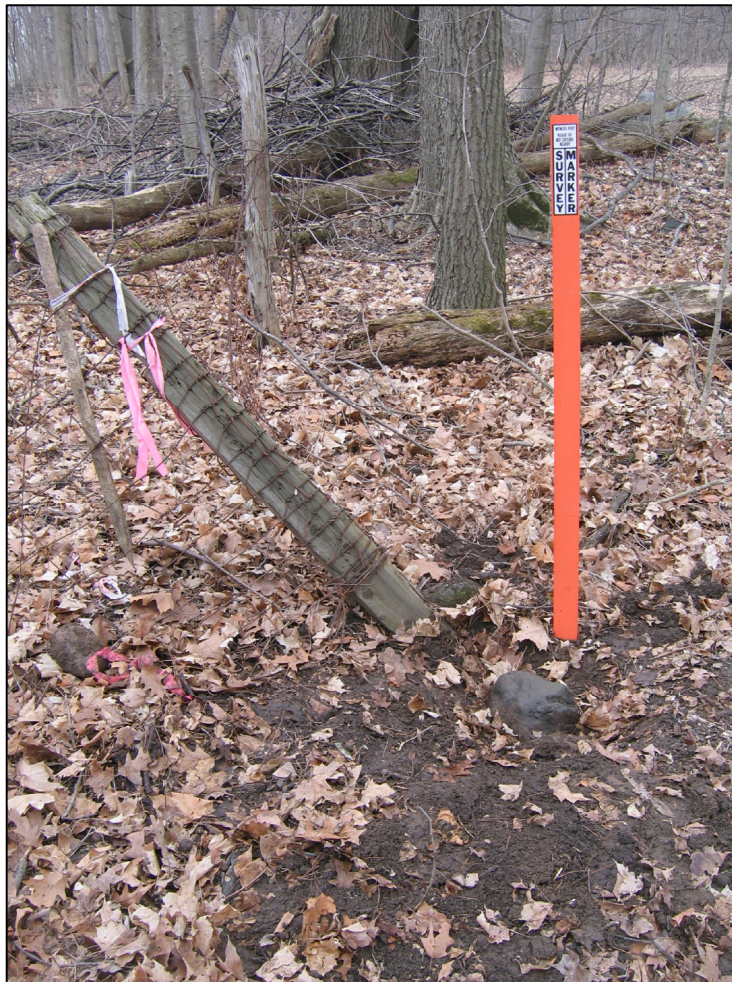
The stone, old wood post and fiberglass witness post. View from the east.
