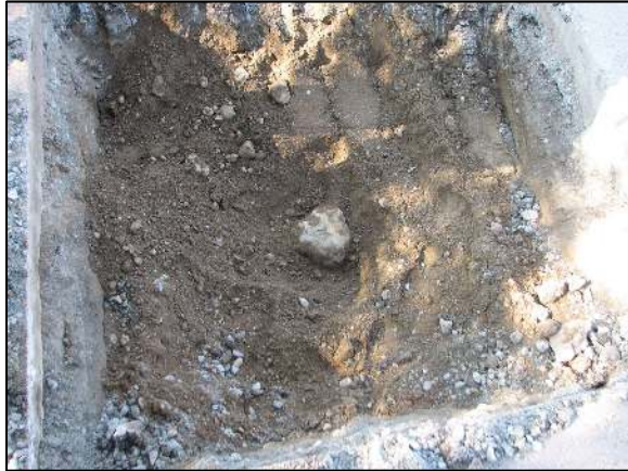
The stone at Corner 1 (Boone County corner) as it was originally exposed.
