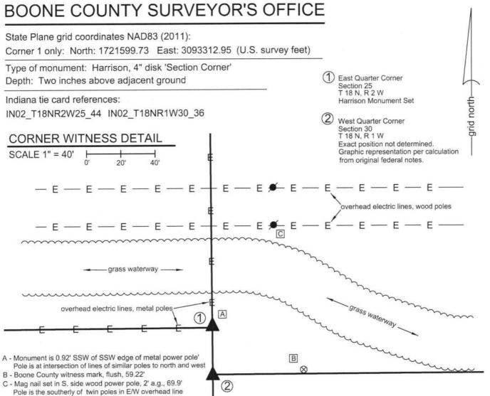
The Harrison monument at Corner 1 was set in the same position as a wood corner post which has been removed. Corner 2 is not an original federal corner and the position of Corner 2 is not firmly established by this document.
