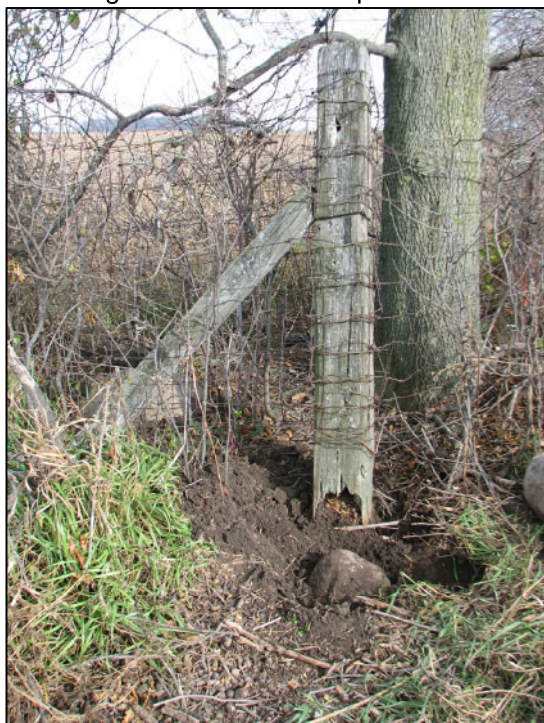
The rock held as marking the corner at the west edge of the base of the post.
