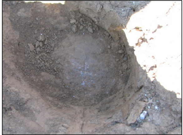
The lower stone at the corner 1/4 mile east. Note the etched "+" mark on top.
