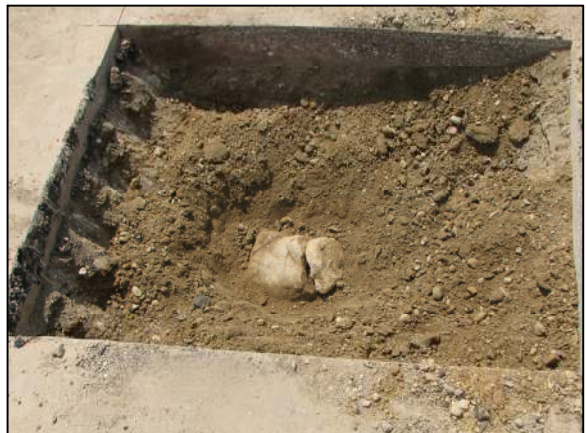
The stone at corner 2, broken due to the fact that the boat spike shown above had been driven into it.
