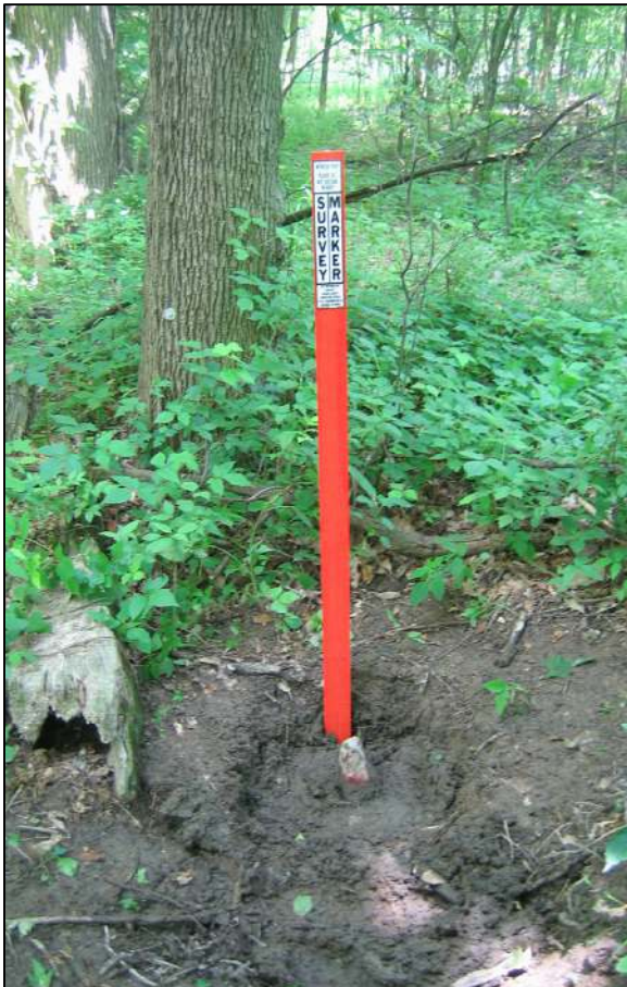
The stone and witness lathe on 6/9/2009.
