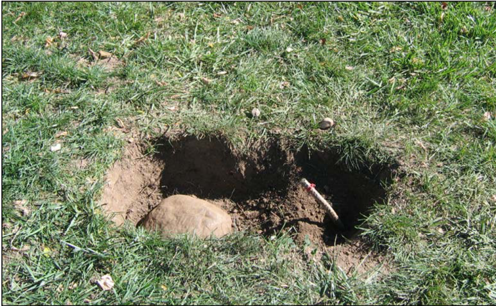
Photo shot from west, showing stone and bent 5/8" rebar.
