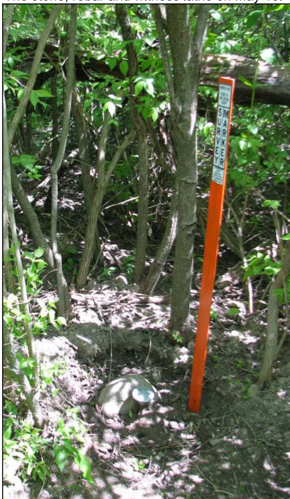
The stone, rebar and witness lathe on May 15.
