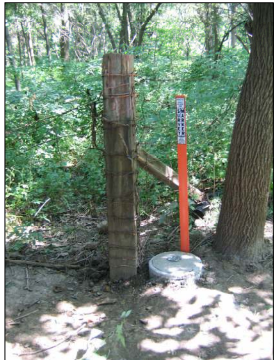
The harrison monument set in place of the stone. Note that the bottom of the post was shifted to the north, see attached notes.
