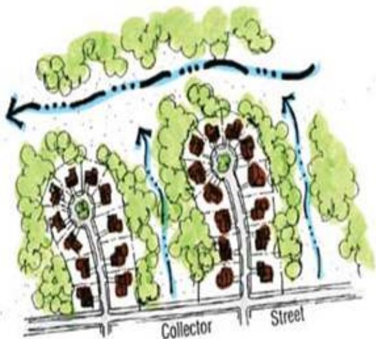
Figure 3 Natural drainage features can guide the design Source: Delaware Department of Natural Resources and Environmental Control - Conservation Design for Stormwater Management
