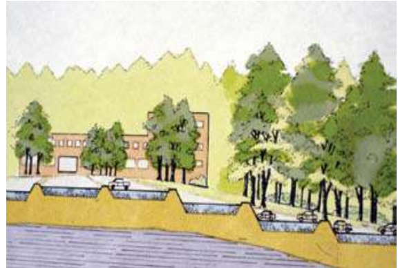
Figure 3 Slope stepping with berms Source: Andropogon
